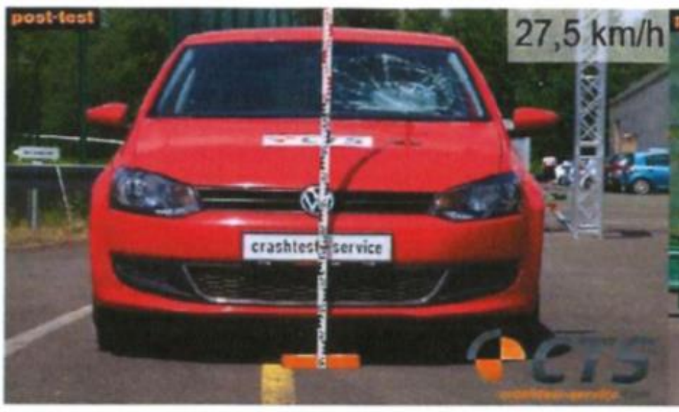
Image 4: Damaged Volkswagen Polo after a test collision with a 'biofidelic' dummy at 17 mph (from the Kortmann Paper).
